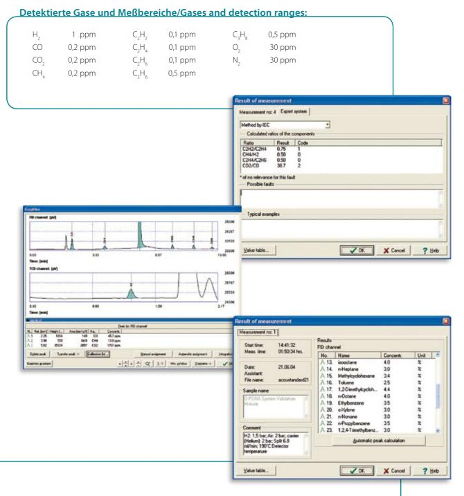
All results are displayed in ppm, the sensitivity is as low as 0,1 ppm for certain hydro-carbons. Therefore, also new transformer oils and transformers after their periodic maintenance can be analyzed.
